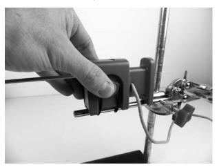
2. Place the fan close to the probe and place a small folded piece of paper towel (about 1 x 4cm) on the tip as shown.
