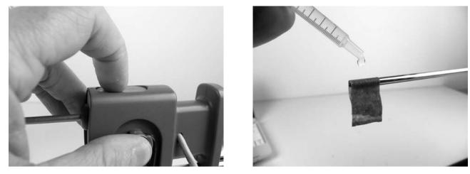
4. Once the temperature no longer falls, stop logging, reset the experiment performing steps 2 and 3 only this time, once the paper has been saturated, place a material sample over the paper as shown. For clarity we have used transparent bubble wrap.
